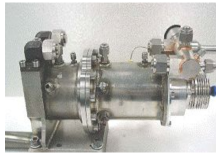
Tubular CPOx reformer
