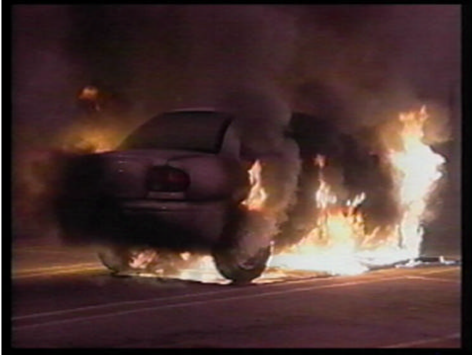
Photo 5 - Time: 2 min, 20 sec - Frame prior to interior deflagration.
