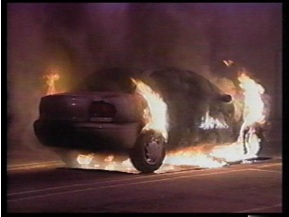
Photo 7 - Time: 2 min, 40 sec - Frame prior to driver's side rear tire rupture.
