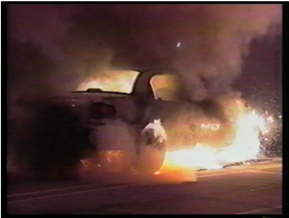
Photo 6 - Time: 2 min, 20 sec - Deflagration in the interior, following frame shows flames exiting around edges of trunk lid.
