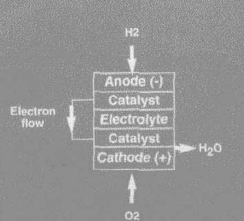
which take different paths to the cathode. The proton passes through the electrons create a separate current that can be utilised before they return to the cathode, to be reunited with the hydrogen and oxygen in a molecule of water.
