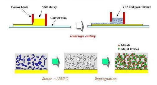
A new procedure was required to fabricate the Cu-based, ceramic-metallic, composite anodes. Because of the relatively low melting temperature of Copper oxides, the ceramic component is manufactured first, typically by tape-casting methods with pore formers. The Cu and catalytic components (primarily ceria) are added in a separate step by wet impregnation.
