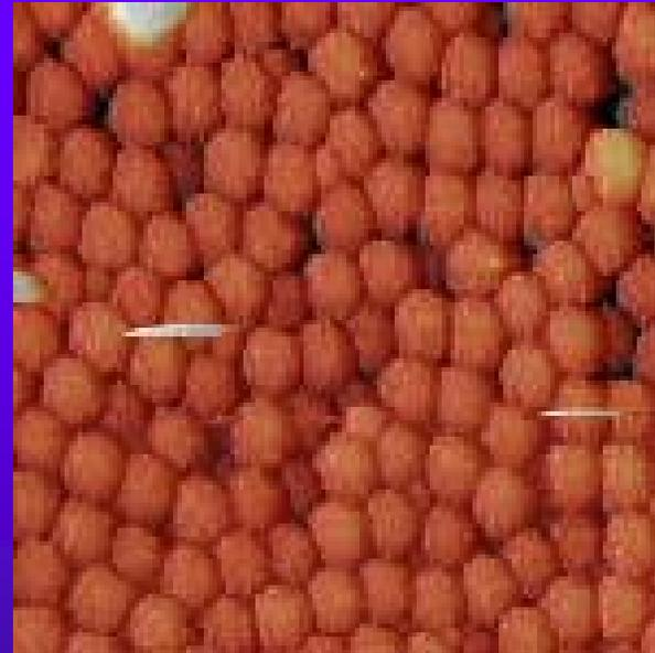
Images of a "raspberry" polymer. Due to the fragile nature of this sample, non contact imaging was the only mode that could be used to successfully scan the sample.
