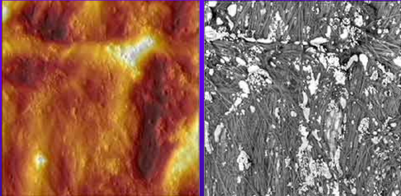
Phase Imaging is quite effective for mapping the sub-micron properties of multi-component polymer systems based on the relative elasticity of individual components.
