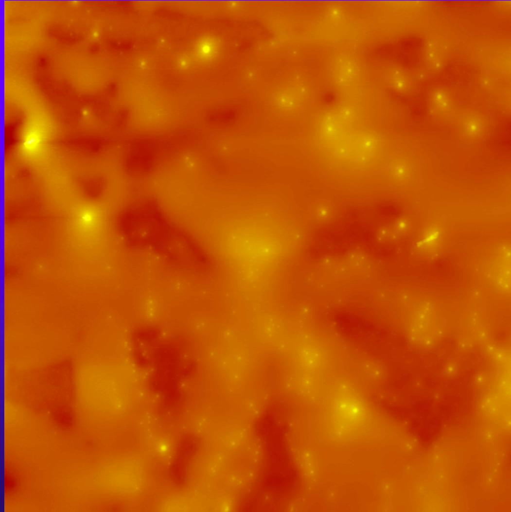
Syndiotactic Polypropylene : 120 Degrees C, With Fading, 40 $\mu$ m Scan
