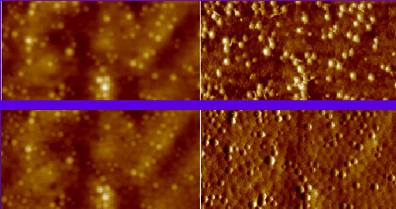
*AFM height (left) and phase (right) images of a two - component latex blend consisting of spheres of about 120nm diameter.*
