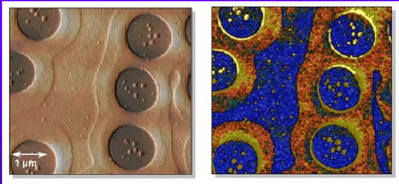
Topography (left) and adhesion (right) images of spin casted polymer (PS/PMMA).
