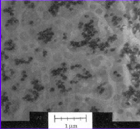
*Transmission electron micrograph of impact-modified plastic containing three components. Differences in the contrast are a consequence of chemical staining of the sample.*
