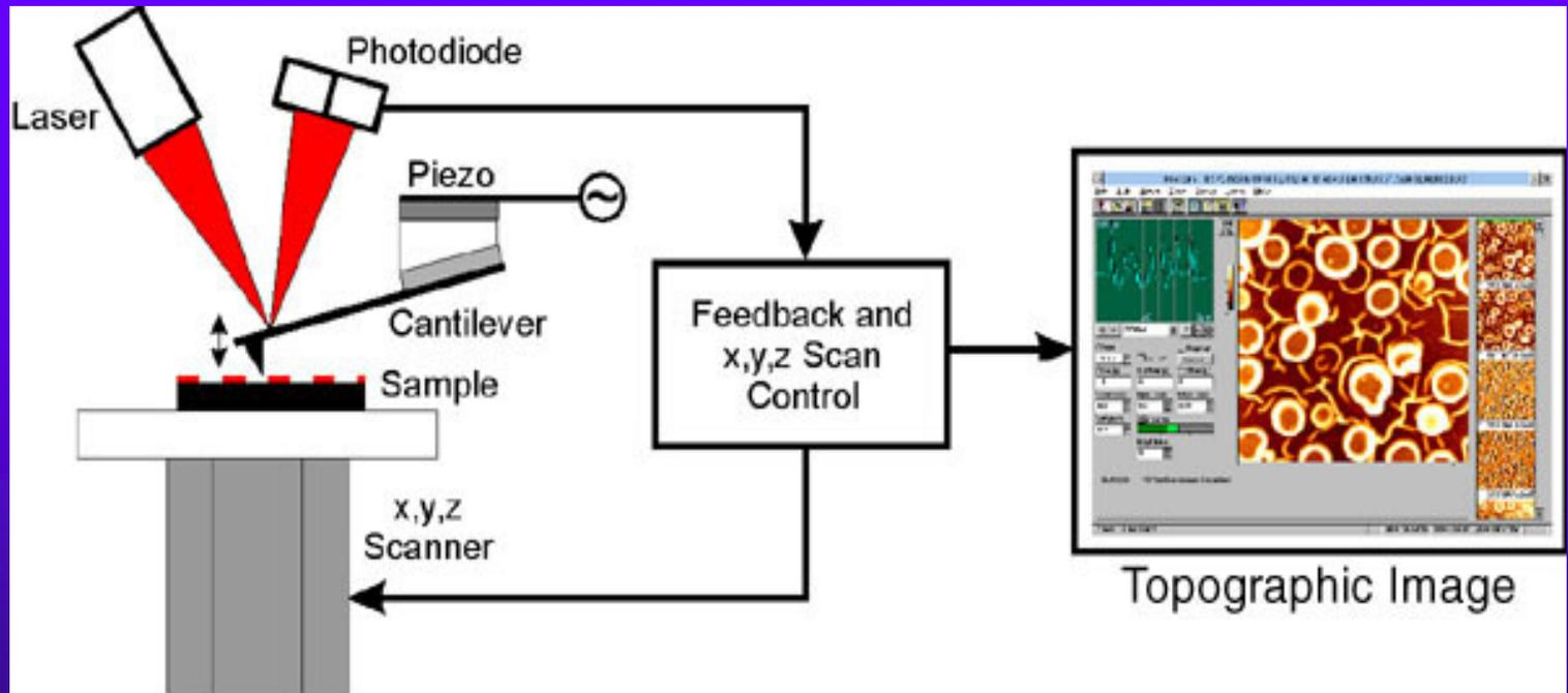
Figure Schematic of an atomic force microscopy (AFM) showing the force sensing cantilever.
