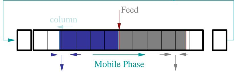
Products are removed by bleeding off a carefully calculated flow at suitable exit points. This changes the velocity of the bands in the column and forces the products to move toward the ports
