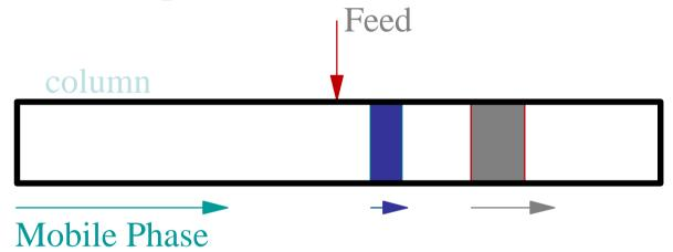
A sample is injected in the centre of a stationary column The two components move at different speeds and are separated
