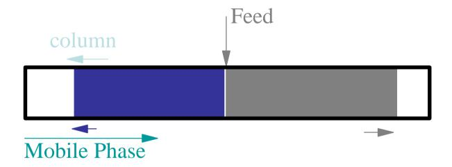
This is clearly a continuous system, but there are problems. It needs an infinite column length and some way to introduce and remove the sample and the products.
