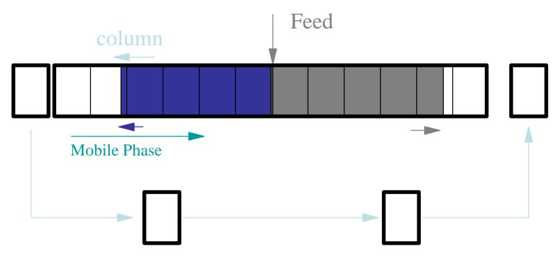
The feed and solvent inlets are now placed between the segments and are moved each time a segment is moved from one end to the other
