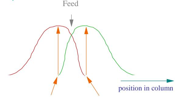
Although the concentration of the solute is low the capacity factor does not take its analytical value The actual value depends on the isotherms and the concentration of the other species.
