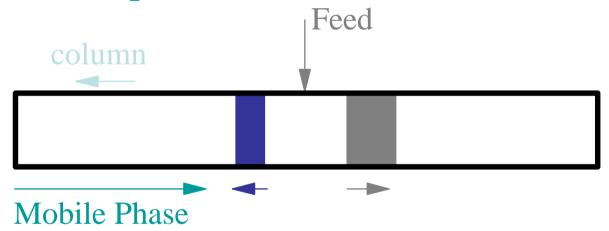
If we now move the column from right to left, at a speed halfway between that of the solutes, they now move in different directions
