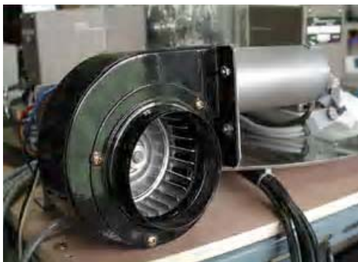
Fig. 11. Heating fan for maintaining column temperature.
