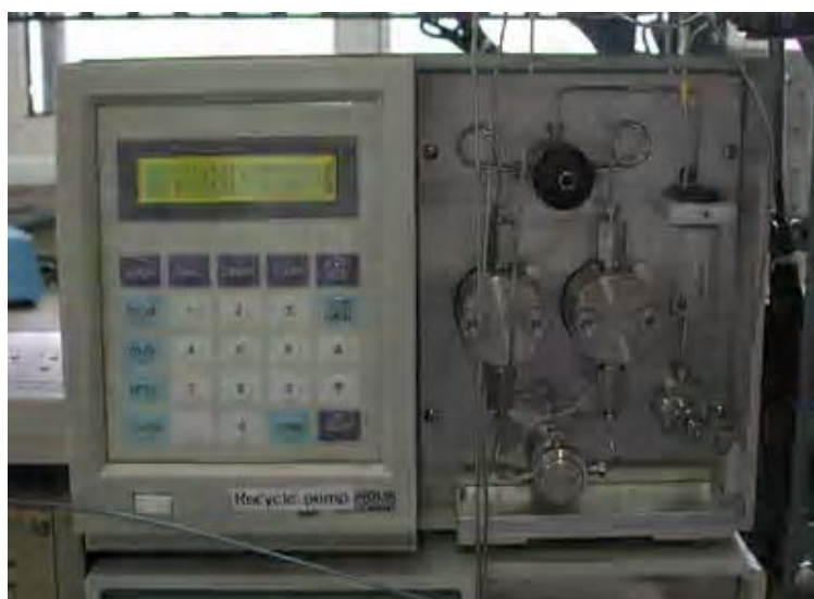
Fig. 7. HPLC pump used in SMB chromatography.
