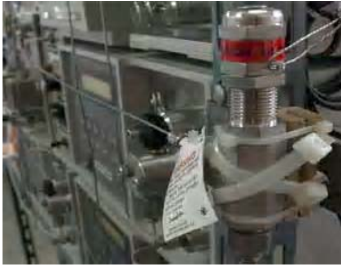
Fig. 9. Pressure relief valves at extract and raffinate port.
