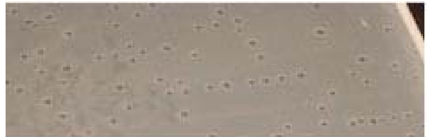
Calcium carbonate nucleating from solution in a Langmuir trough at NLS beamline X22B.
