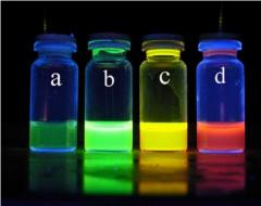
CdSe quantum dot fluorescence showing an increase in dot size going from green on the left to red on the right.
