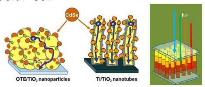
Electron transport through a structure of nanoparticles (left) and more ordered nanotubes (center) is shown. At right, different wavelengths of light can be absorbed by different-sized quantum dots layered in a "rainbow" solar cell
