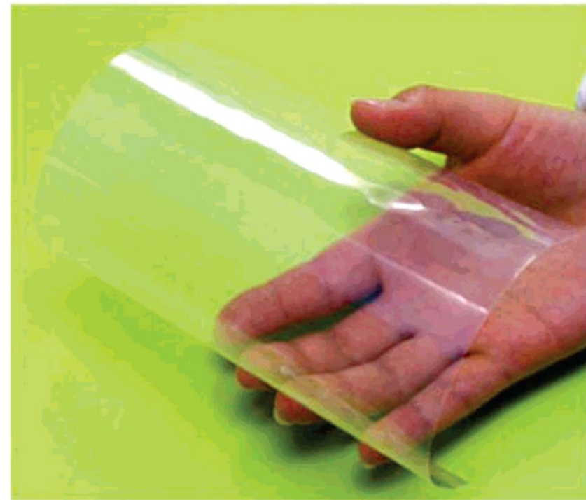
Fig. 7. Appearance of optically transparent acetyl BC nanocomposite.
