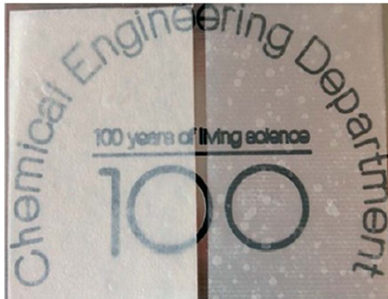
Fig. 2 Comparison of the transparent papers made from BC (left) and MFC (right). Reprinted with permission from K. Y. Lee, T. Tammelin, K. Schultzer, H. Kiiskinen, J. Samela, A. Bismarck, High performance cellulose nanocomposites: comparing the reinforcing ability of bacterial cellulose and nanofibrillated cellulose, ACS Appl. Mater. Interfaces, 2012, 4(8), 4078–4086.
