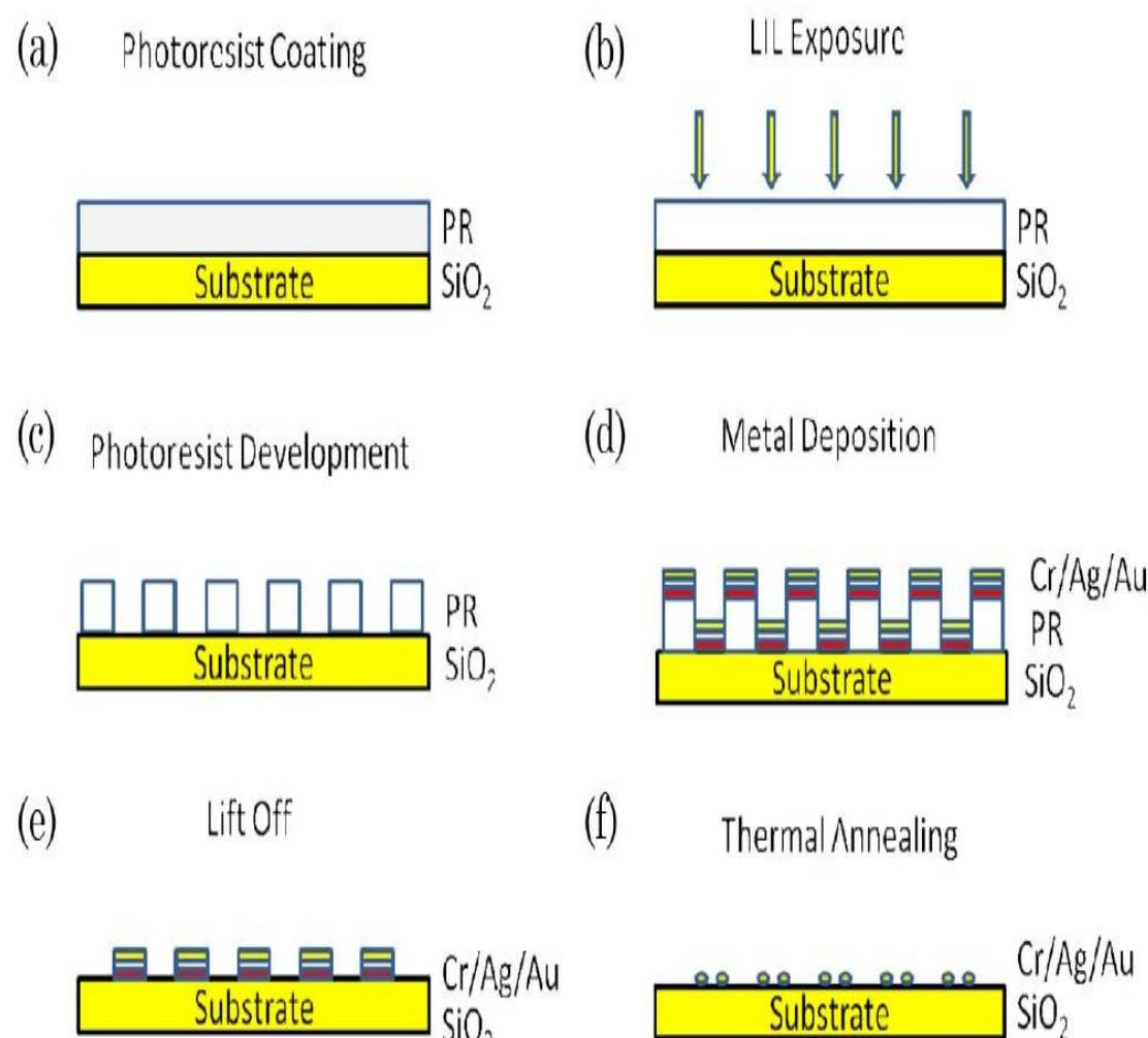
Fig. 1. (Color online) Fabrication of Ag/Au bimetallic nanodots arrays by LIL and thermal annealing: (a) PR spin coating; (b) PR exposure by LIL; (c) PR developing; (d) Cr, Ag, and Au metallic thin film deposition; (e) lift-off; and (f) thermal annealing.
