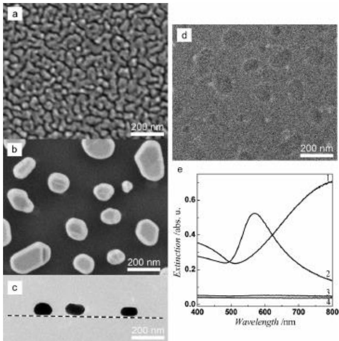
FIG. 1. HRSEM (a,b,d) and cross-sectional TEM (c) images of 10 nm (nominal thickness) Au island films on cover-glass substrates: a) as-evaporated; b,c) after annealing 10 h at 550 °C; d) after island dissolution in aqua regia. The transmission UV-vis spectra in (e) correspond to: 1, a; 2, b; 3, d; 4, bare glass. The line in (c) is drawn as
