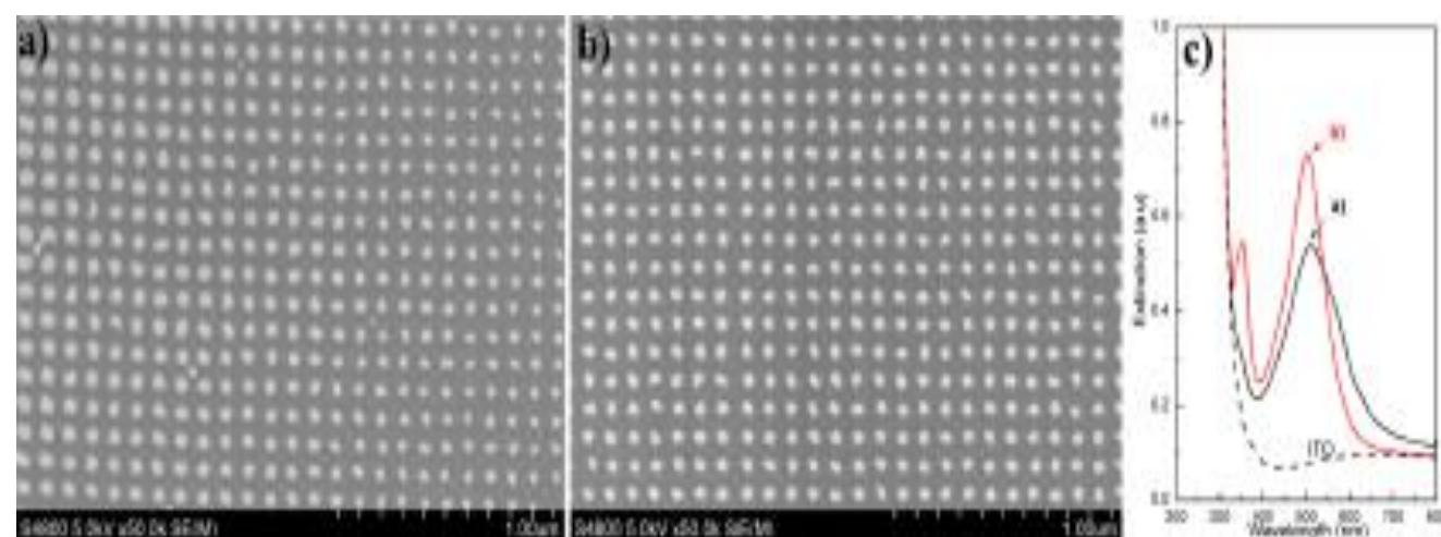
Fig. 2 Top-view SEM images of Ag nanoparticles fabricated on ITO glass using a UTAM template prepared (a) with and (b) without PMMA as the supporting layer. (c) UV-vis extinction spectra of ITO glass and samples shown in (a) and (b) (the strong absorptions below a wavelength of 320 nm in both spectra are associated with the optical band gap of ITO glass).
