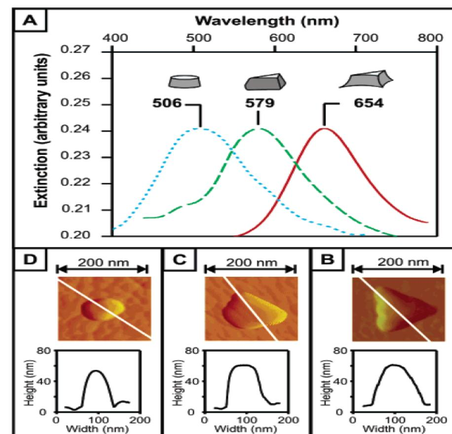
FIG. 2. LSPR spectra and AFM images of Ag nanoparticles on ITO. (A) LSPR of the Ag nanoparticles. (B) AFM image before any electrochemical measurements. (C) AFM image after one measurement. (D) AFM image after two measurements.
