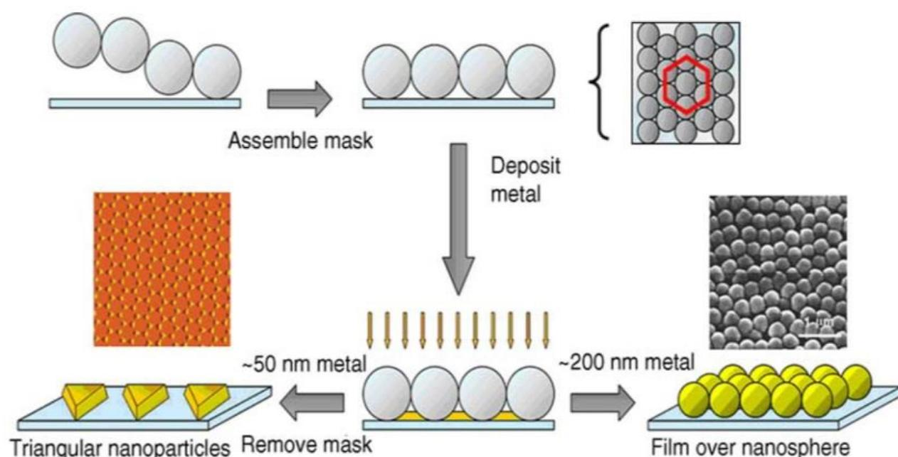
FIG. 1. Schematic illustration of the nanosphere lithographic fabrication of nanoparticle arrays (left side) and film over nanosphere surfaces (FON; right side) and corresponding micrographs. [Talanta 67 , 438–44892005)]
