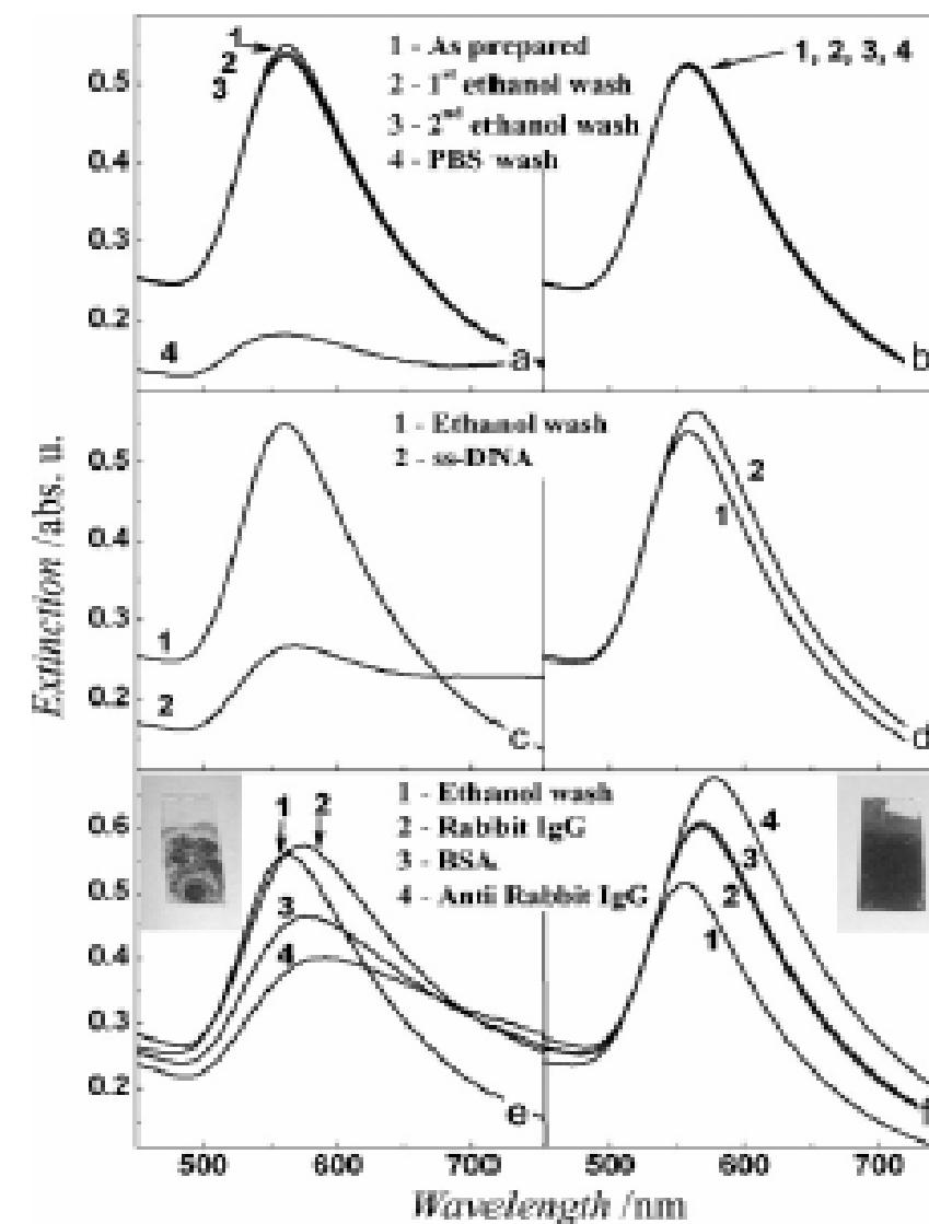
FIG. 2. Transmission UV-vis spectra of 10 nm Au island films on cover-glass, annealed 10 h at 500 °C (a,c,e) and at 550 °C (b,d,f): a,b) after washing in ethanol (2 times) and PBS solution; c,d) self-assembly of a ss-DNA monolayer; e,f) protein–protein (antigen–antibody) recognition experiments. In (c–f) the first spectrum shown is after ethanol wash. Insets in (e,f): photographs showing the corresponding samples after the entire treatment sequence.
