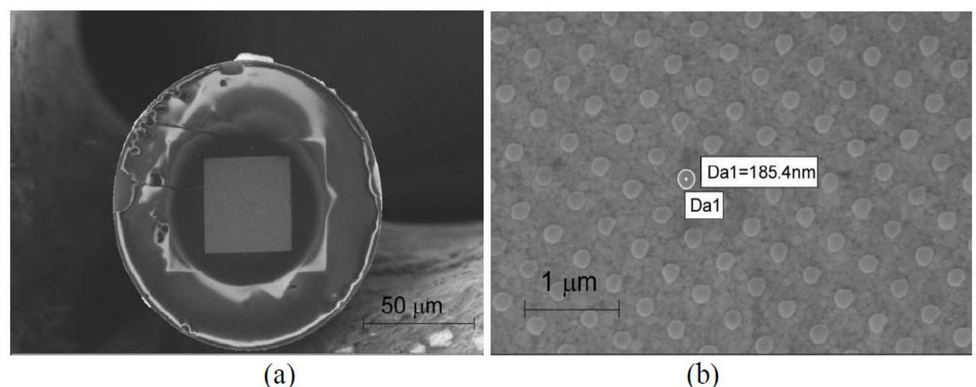
FIG. 2. Scanning electron micrographs of a gold nanodot array on an optical fiber tip. (a) Overview of the optical fiber end facet, and (b) gold nanodot array on the optical fiber facet.
