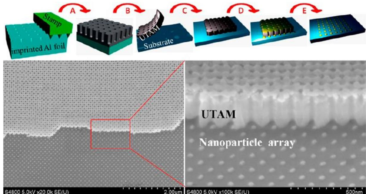
Fig. 1 Schematic outline of the fabrication processes for highly ordered nanoparticle arrays by combining nanoimprinting with UTAM technique (processes A to E are anodization of prepatterned Al foil, removal of backside Al and barrier layer and pore-widening, mounting the UTAM on the substrate, deposition of materials, and removal of UTAM, respectively). SEM images of Au nanoparticle arrays after totally removing the UTAM.
