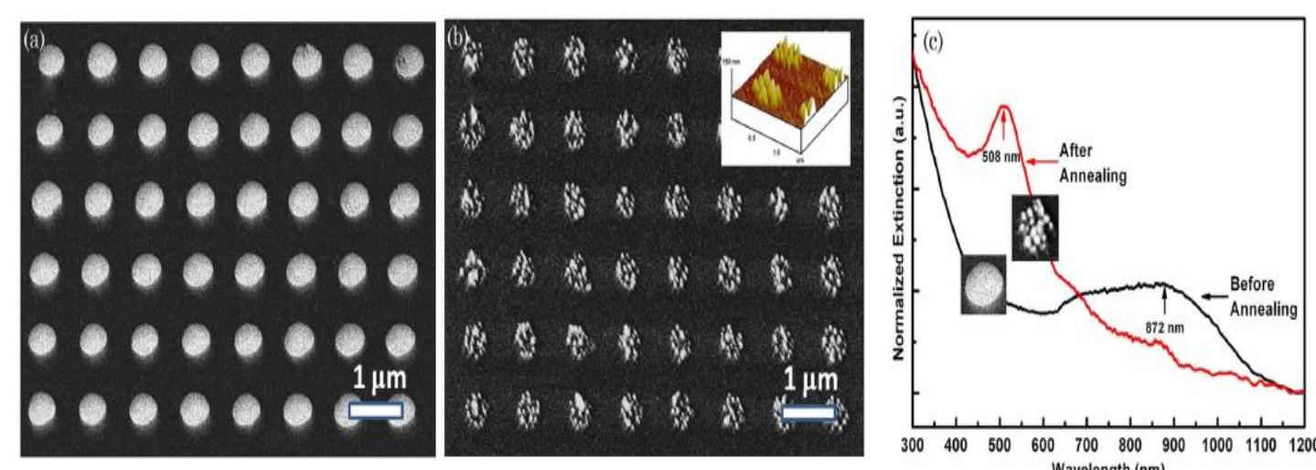
Fig. 2. (Color online) SEM images of  $\text{Ag}_{0.75}\text{Au}_{0.25}$  bimetallic nanodisk arrays fabricated by LIL (a) before and (b) after thermal annealing, and (c) their measured extinction spectra.
