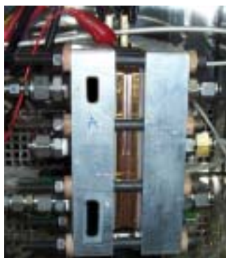
Figure 1. 240\text{cm}^2 single cell using the SUS316 plates.
