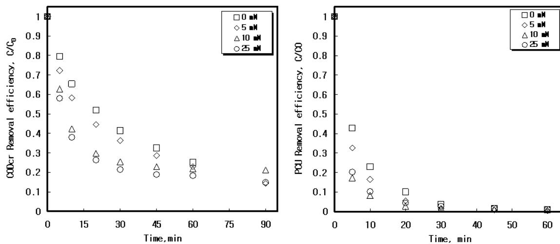
Fig. 3. Effect of  $\text{H}_2\text{O}_2$  concentration on the organic and color removal efficiency at  $\text{UV}/\text{O}_3/\text{H}_2\text{O}_2$  system.
