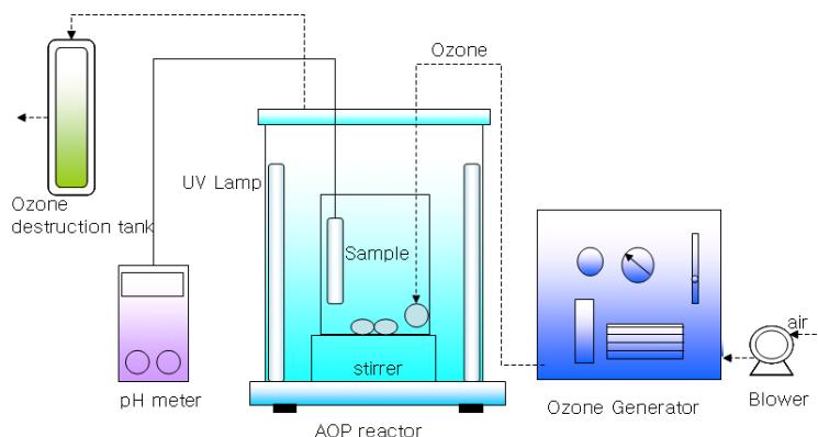
Fig. 1. Schematic diagram of AOP equipment.
