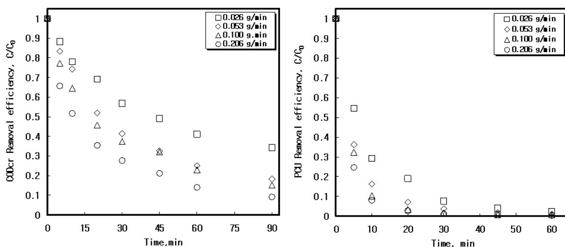
Fig. 2. Effect of ozone concentration on the organic and color removal efficiency.
