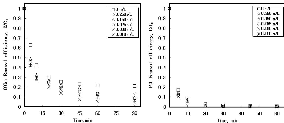
Fig. 4. Effect of  $\text{FeSO}_4$  dosage on the removal of organic and color at  $\text{UV}/\text{O}_3/\text{H}_2\text{O}_2/\text{FeSO}_4$  system.
