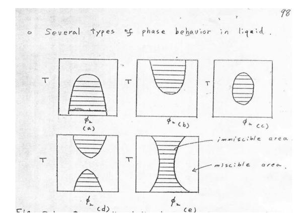
Fig. Schematic of liquid - liquid temperature - composition phase diagrams.
