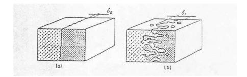
Fig.34 Model of the interphase layer in a polyolefin blend (a) after dispersive mixing: (b) after laminar mixing and/or heat treatment (Courtesy Yu. S. Liparov
