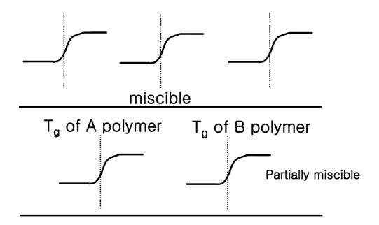
shifted toward center by DSC (differential scanning calorimeter) measurement .
