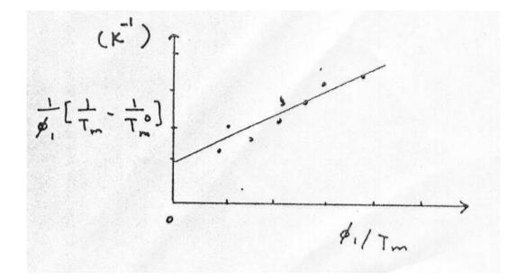
e.g) PVF2-PMMA blend  $\chi_{12}$  = -0.295 at 160 °C ref.) Olabisi et. al. , Polymer- Polymer Miscibility
