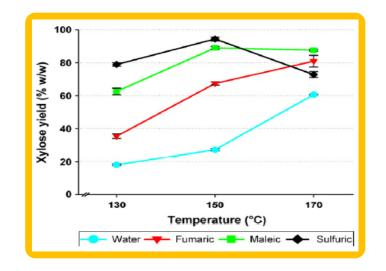
Fig. 3. Xylose yield as function of pretreatment temperature, measured after enzymatic hydrolysis (72 h, 50 °C). 100% = 0.21 g xylose/g dry matter straw. Error bars represent standard deviation.
