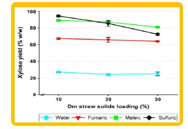
Fig. 6. Xylose yield as function of dm straw loading, with equal acid:straw ratio, measured after pretreatment. Pretreatment temperature 150 °C. 100% = 0.21 g xylose/g dry matter straw. Error bars represent standard deviation.
