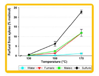
Fig. 4. Furfural formation from xylose as function of pretreatment temperature. Error bars represent standard deviation.
