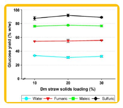
Fig. 5. Glucose yield as function of dm straw loading, measured after enzymatic hydrolysis (72 h, 50 °C). Pretreatment temperature 150 °C. 100% = 0.40 g glucose/g dry matter straw. Error bars represent standard deviation. • Raising the solids loading in the pretreatment would decrease process cost, both by lowering reactor size and heating requirements during the pretreatment.
