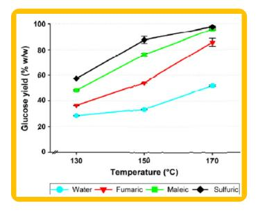
Fig. 1. Glucose yield as function of pretreatment temperature, measured after enzymatic hydrolysis (72 h, 50 °C). 100% = 0.40 g glucose/g dry matterstraw. Error bars represent standard deviation.
