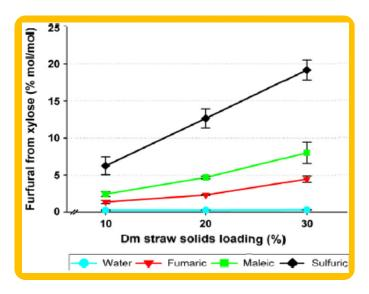
Fig. 8. Furfural formation from xylose as function of dm straw loading. Pretreatment temperature 150 °C. Error bars represent standard deviation. • after sulfuric acid pretreatment, enzymatic xylose yield decreased by more than 20%. This was largely caused by formation of ca. 15% more furfural (Fig. 8).
