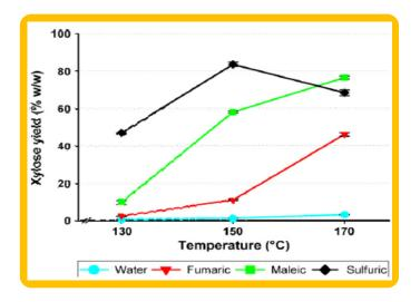
Fig. 2. Xylose yield as function of pretreatment temperature, measured after pretreatment. 100% = 0.21 g xylose/g dry matter straw. Error bars represent standard deviation.
