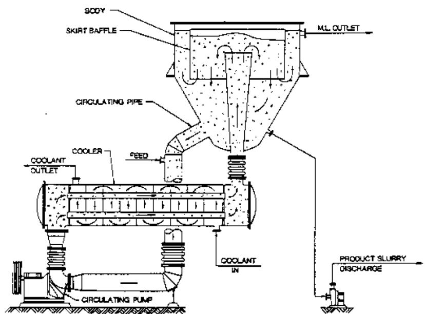
Fig 17. Swenson surface cooled Crystallizer
