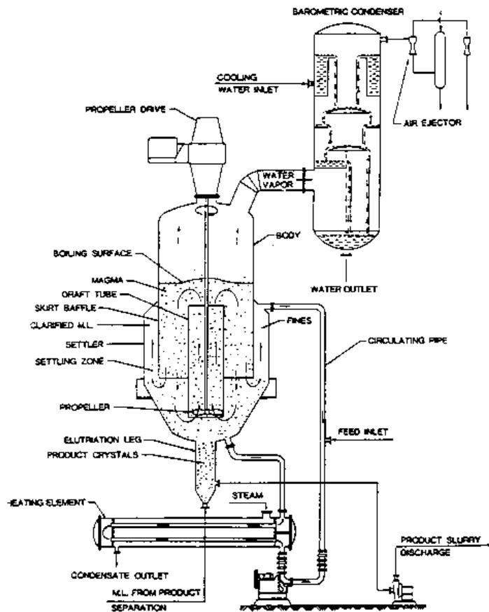
Fig 16. Swenson draft tube baffle Crystallizer
