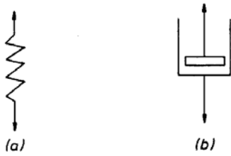
Fig. 3.2 Diagrammatic representations of ideal rheological behaviour: (a) The Hookean spring; (b) The Newtonian dashpot.
