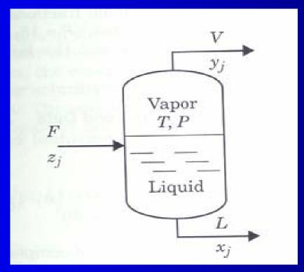
The evaporator will operate under high pressure, between 15 and 25 atm with a feed stream at 50°C
