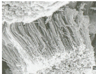
TiO 2 nanowires from its sol-alumina removed
