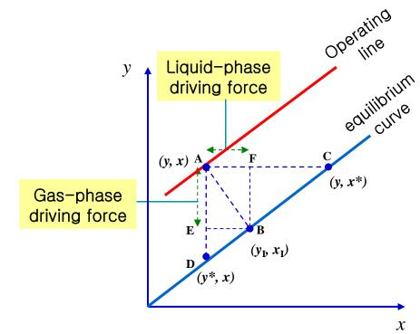
Rate of mass transfer can be increased by promoting turbulence and/or increasing dispersion
