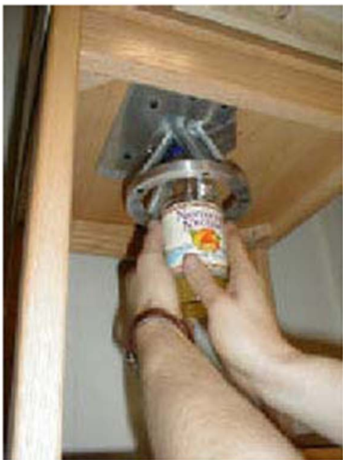
Easy Jar Opener: Attaches below upper kitchen cabinets, grip jar with two hands and twist cap off easily.
