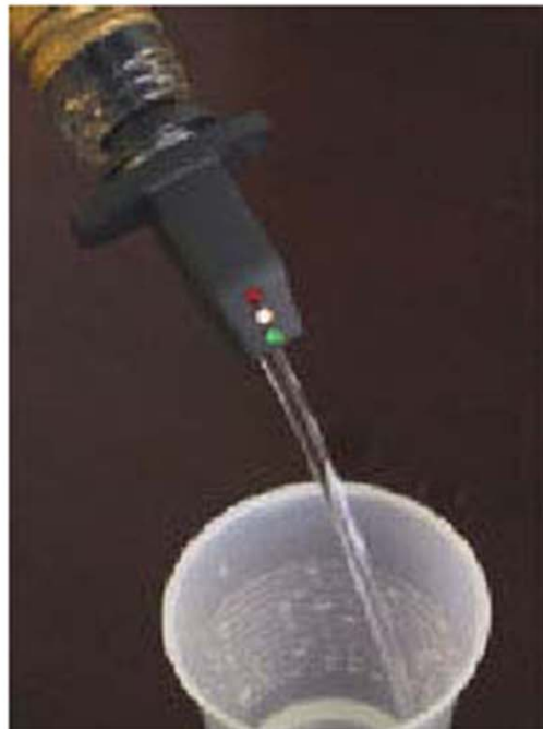
Bartender's Pour Spout: Times the pouring of liquor drinks, green-yellow-red LED light sequence shows when one shot is poured.
