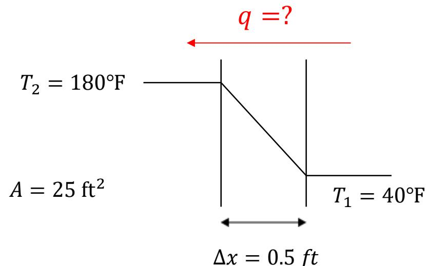
$$k = \begin{cases} 0.021 \text{ Btu/ft} \cdot \text{hr}^{\circ}\text{F} @ 40^{\circ}\text{F} \\ 0.032 \text{ Btu/ft} \cdot \text{hr}^{\circ}\text{F} @ 180^{\circ}\text{F} \end{cases}$$
