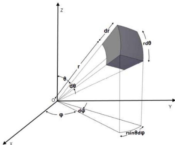
$$q_{\text{in}} - q_{\text{out}} + \dot{q} = \frac{\partial(mC_p T)}{\partial t}$$
