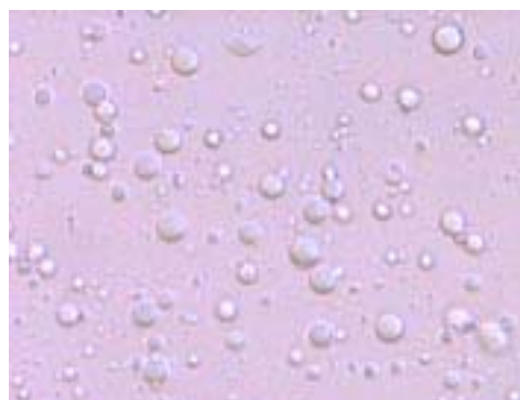
Figure 2. Optical image of W/O emulsion prepared by adding HPC polymer
