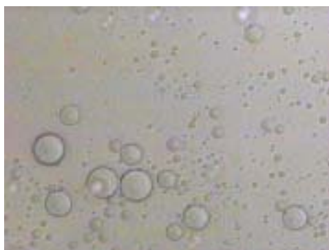
Figure 1. Optical image of W/O emulsion prepared by Tween20 and Span80
