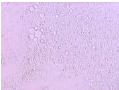
Figure 3. Optical image of W/O emulsion prepared by adding PEG polymer
