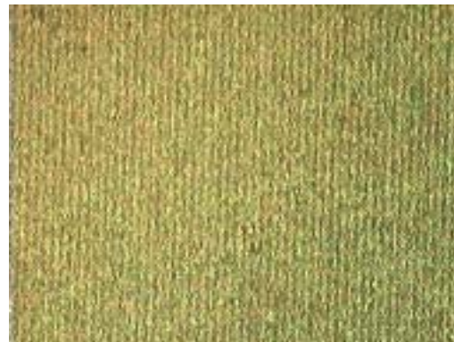
(c) Optical microscope photograph of \text{Ag-SiO}_2 gratings surface after annealing 600^\circ\text{C}
