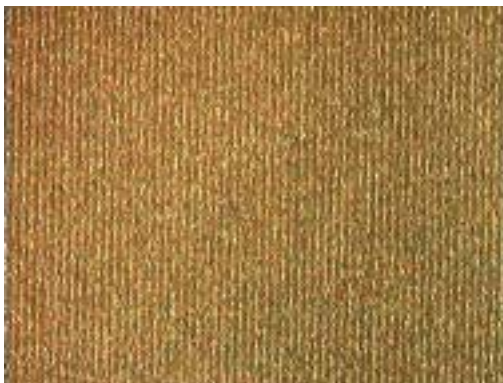
(b) Optical microscope photograph of \text{Ag-SiO}_2 coatings exposed to Ar-ion laser
