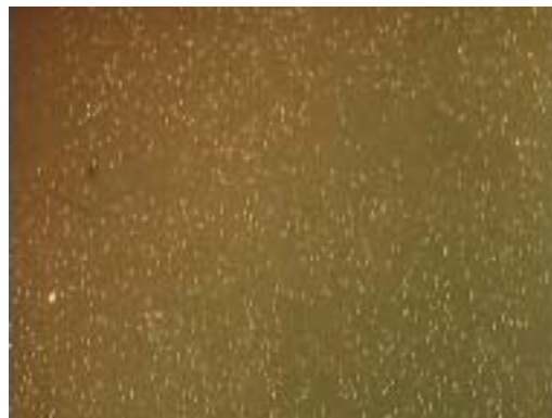
Fig 4. (a) Optical microscope photograph of \text{Ag-SiO}_2 Coating surface
