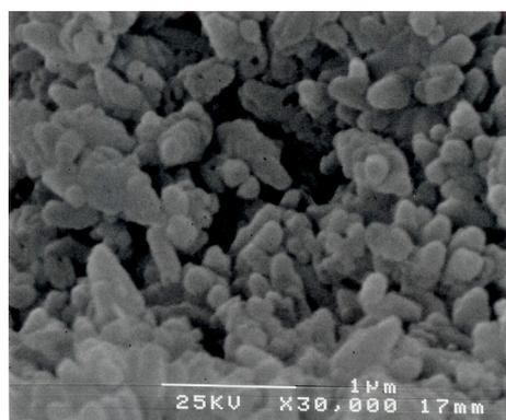
100% H<sub>2</sub>O(500ml) + Ca(OH)<sub>2</sub>(30g) +CO<sub>2</sub> gas(1l/min)
