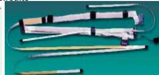
Headliner harness utilizing flat wire
