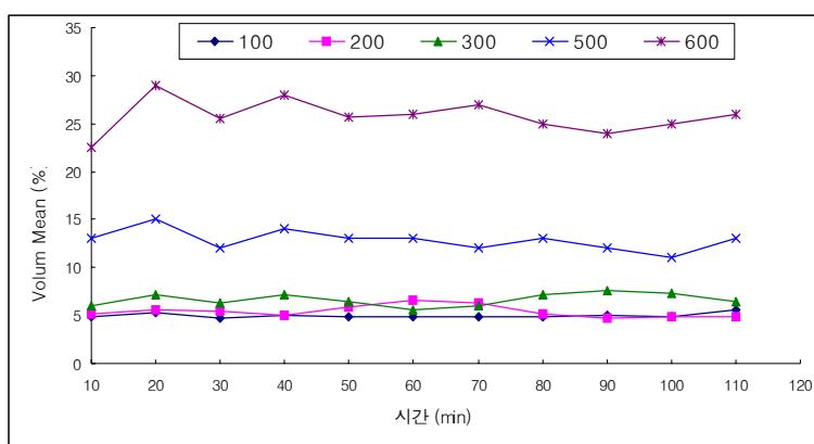
Fig. 3 Volume mean size change by the RPM.
