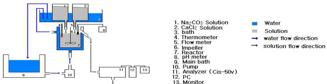
Fig. 2 schematic diagram of experiment.
