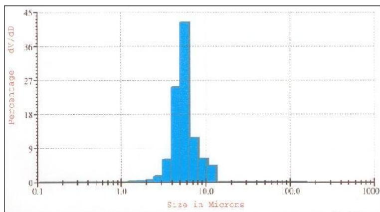
Fig. 5 CSD of the calcium carbonate crystals after startup 180 min.
