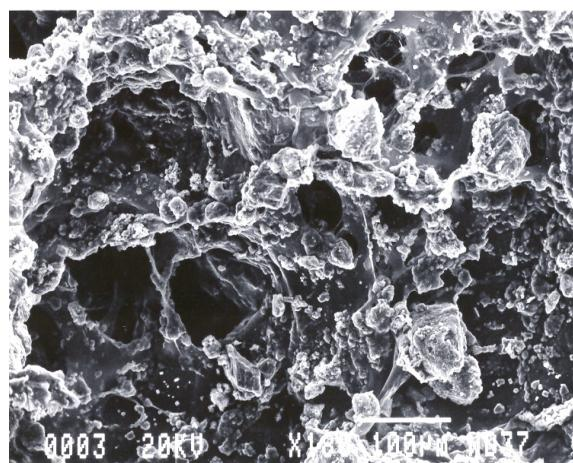
Figure 1. SEM photograph of the surface of waste lime support carrier.
