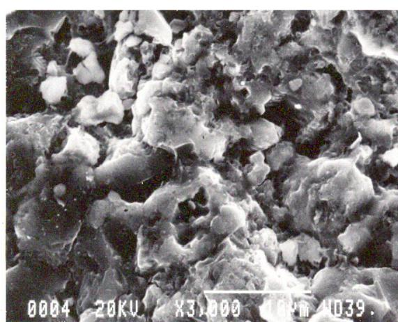
Figure 2. SEM photograph of the interior of support carrier after immobilization.
