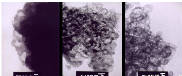
Figure 1. TEM image of hollow silica particle; spherical particle by \text{CaCO}_3 template. (molar ratio of \text{SiO}_2/\text{CaCO}_3 = 1/3, 1/7.5, 1/10 )
