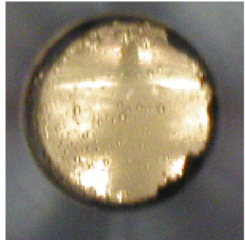
Fig. 2. Photographic image of copper bath containing 10 vol% supercritical CO 2 at 15 MPa and 25°C.
