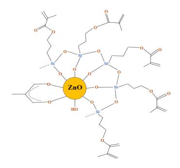
Proposed structural model of surface modified ZnO QDs after synthesis.
